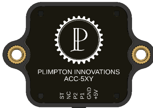
Figure 2: Acceleration Sensor Backing Plate with Nomenclature.
